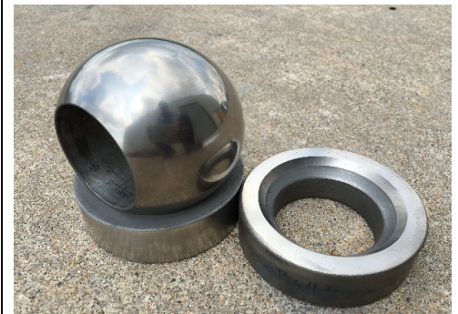
Ball and seat valve coated, finish ground and lapped.
