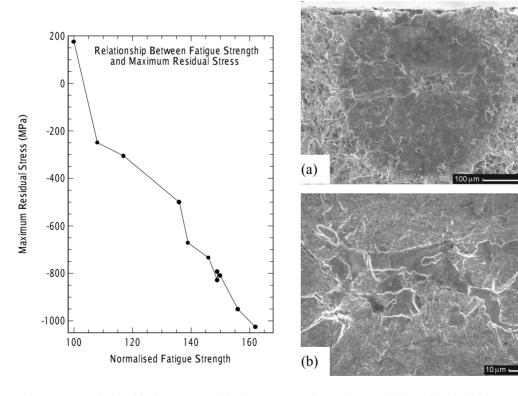
Figure 5 Relationship between residual Stress and fatigue strength.
