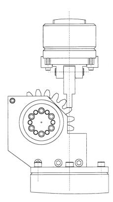
Figure 2 Gear pulsator test method.
