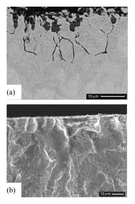
Figure 1 (a) Section with internal oxidation. (b) Surface initiated fracture.
