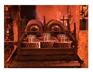
Figure 1: Load of Production Gears (650 lbs net) in Position for Loading into an Atmosphere Carburizing Furnace followed by Oil Quenching.
