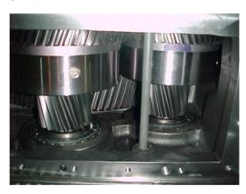
Figure 4: Heavy Duty Marine Transmission Transfer Gears.
