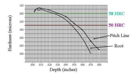
Figure 7: Pitch Line & Root Comparison: Vacuum Carburized (High Gas Pressure Quenched) Gear
