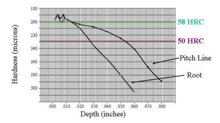
Figure 5: Pitch Line & Root Comparison: Atmosphere Carburized (Oil Quenched) Gear
