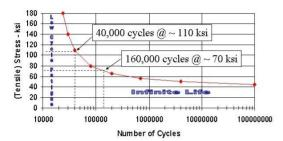
Figure 8: Stress versus Load Cycles
