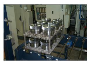
Figure 2: Load of Production Gears (650 lbs net) in Position for Loading into a Vacuum Carburizing Furnace followed by High Gas Pressure or Oil Quenching
