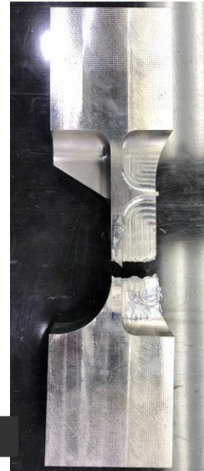
Combined Stress from Applied Load and LSP Residual Stress
