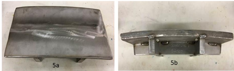
Figure 2. 5a. Canister test panel welded across width. 5b. Side-on view shows stiffening ribs used to help prevent straining as would be the case in the constraint of a canister
