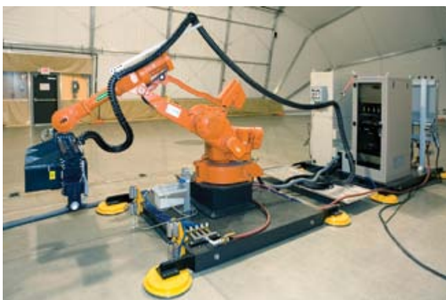
Figure 2. Mobile beam delivery system. The dual-gimbal stinger (DGS) is held by a robot arm. The entire assembly can be freely moved around the processing cell on air bearings. High speed gimbals maintain the optical path between the laser system and the DGS.
