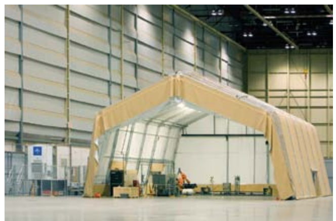
Figure 3. Laser safety tent used for the peening of F-22 fighter jets. The transportable laser system can be seen just to the left of the tent and the mobile beam delivery system is visible inside.
