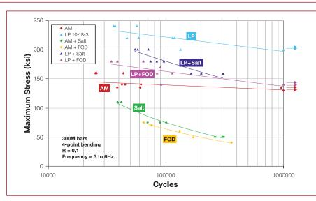
Figure 4. Stress-lifetime curve for laser peened and as machined samples damaged by a 0.020-inch notch cut into the high stress region of the sample using an EDM wire or corrosion simulated by alternate exposure to a 3.5% salt bath. The lack of surface compressive stresses results in rapid deterioration of the AM samples whereas the laser peened samples show more than 250% advantage in fatigue strength.
