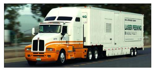
The Mobile Laser Peening Facility contains a fully equipped peening system that can be set up at field sites in less than one week, then dis-assembled and made ready for transport to another site in approximately two days.
