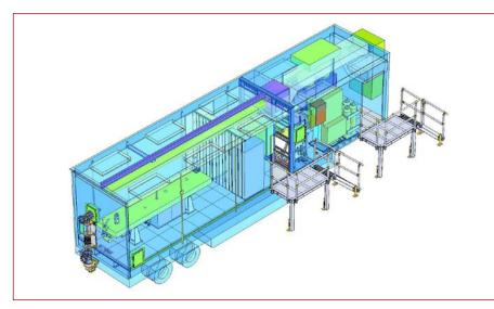
Figure 7. The laser peening system has been packaged into a transportable system for remote processing applications. Requiring only electrical power, a fully equipped peening system can be rapidly set up at field sites for overhaul and repair work.
