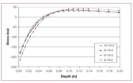
Figure 2. Compressive stress developed by laser peening in 300M in a 0.5-inch-thick sample not corrected for sample bending.
