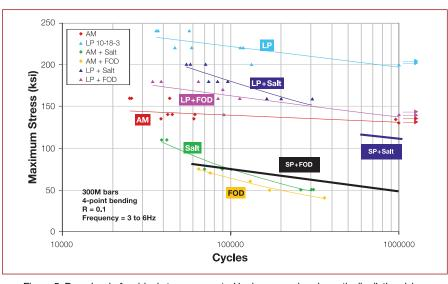
Figure 5. Deep level of residual stress generated by laser peening dramatically distinguishes it from shot peening in the presence of damage such as FOD or salt corrosion.
