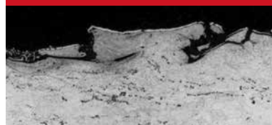
Fig. 11-2B Typical Surface from Proper Media
