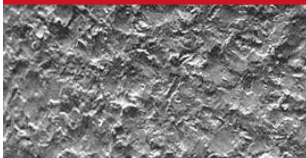
Fig. 10-13 SEM Photo of Dual Peen Surface Finish
