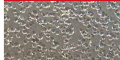
Fig. 11-8B Incomplete Shot Peening Coverage
