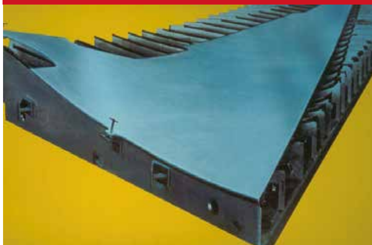
Fig. 10-2 Checking Fixture for Verifying Peen Forming of Wingskin
