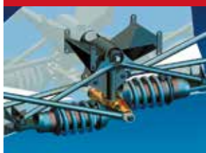
Fig. 5-2 Compression Spring Assembly
