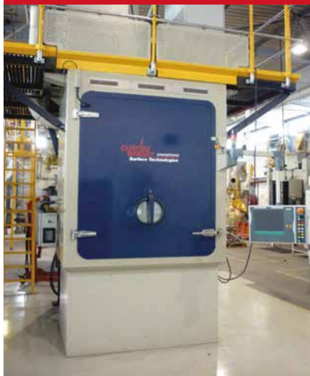
Fig. 11-10B Multi-Nozzle Computer Monitored Shot Peening Machine
