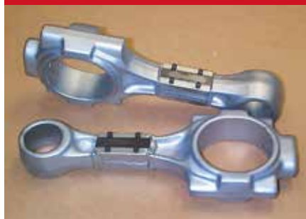
Fig. 11-6 Almen Strip Mounting Fixture
