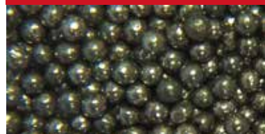
Fig. 11-3B Poor Quality Shot Peening Media
