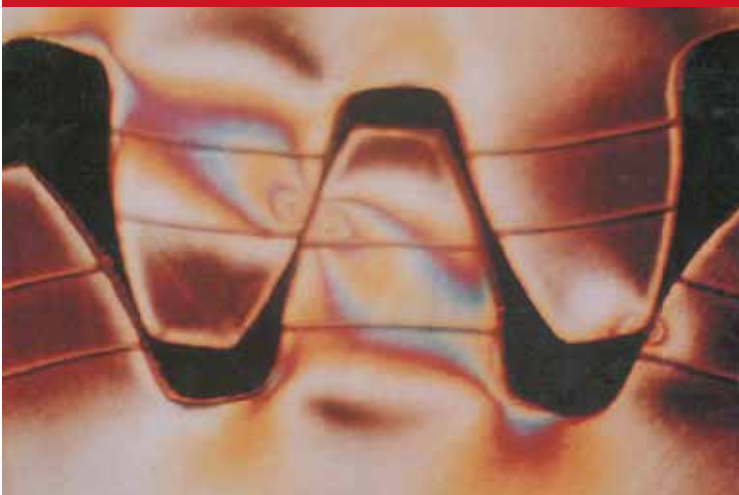
Fig. 4-3 Polarized View of Applied Gear Stresses
