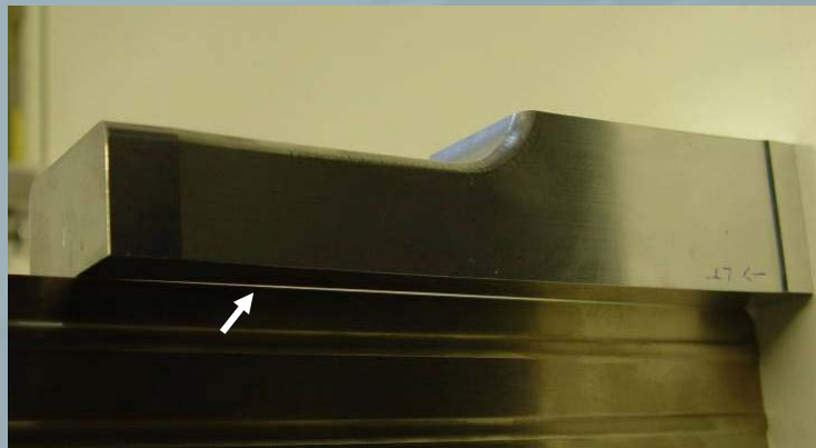
Distortion due to residual stresses (specimen 2b)
