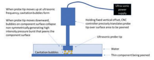
Nonsymmetric collapse of cavitation bubbles creates intense water jet with locally yielding pressure that peens the component surface.
