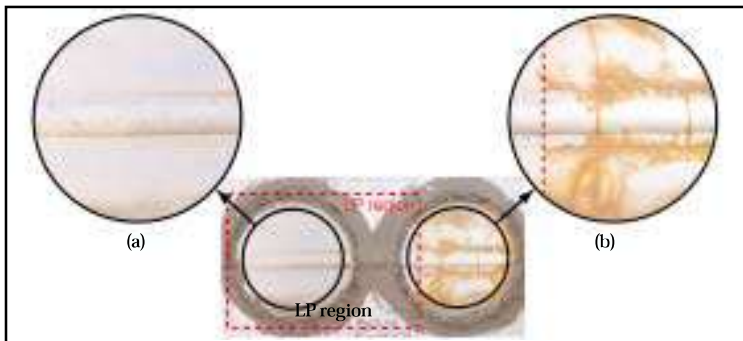
Fig. 3 — Photograph of 316 stainless steel weld tested in boiling MgCl_2 solution, showing (a) no SCC damage on the laser peened section, and (b) extensive SCC damage on the unpeened section, with crack arrest near the boundary of laser peening (red dashed line).
