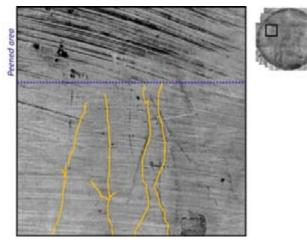
Test plate of 316L stainless steel fabricated by Holtec with stress corrosion cracks highlighted. Observation was done after 57.5 hours exposure to MgCl<sub>2</sub> at 155°C. Cracks developed in un-peened areas, but did not develop in peened areas and arrested as they propagated from un-peened into peened areas.
