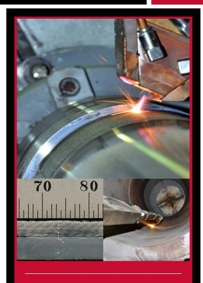
LASER WELD CLADDING
