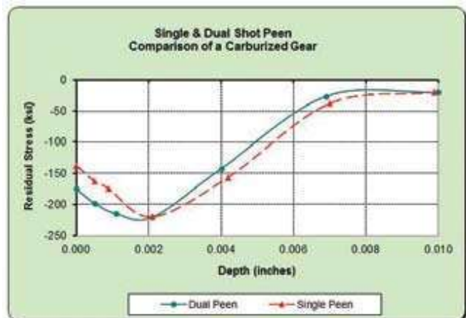
Figure 3. Single and Dual Shot Peen Comparison of a Carburized Gear
