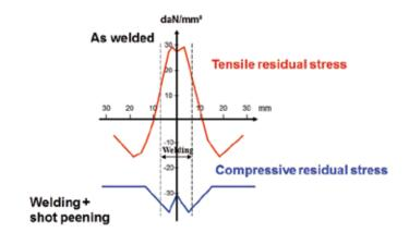
Construction steel E460; TIG welded
