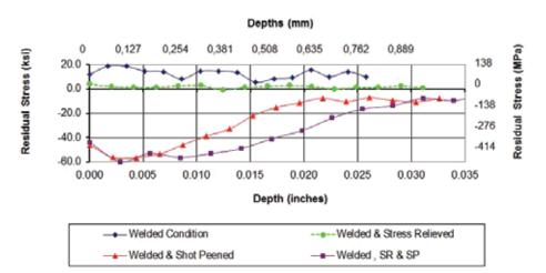
1020 (C22E) Material: BRN 150–180; Rb 80-90 Welded Filler Rod: 7018 – 3/32" Shot Peening: MI-460H @ 16-20A
