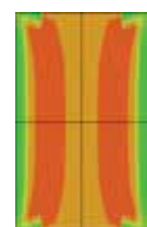
With laser peening – Peak axial stress is 924 MPa
