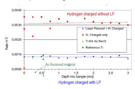
Laser peened with hydrogen charged sample contains 1/3 the hydrogen concentration compared to hydrogen charged sample without laser peening
