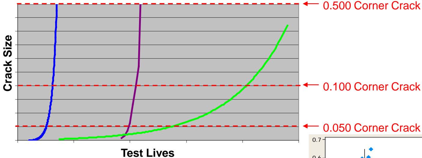
Fitted Crack Growth Data
