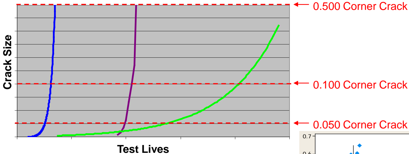
Fitted Crack Growth Data
