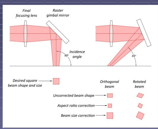
Each pulse is individually corrected for size, rotation, and aspect ratio
