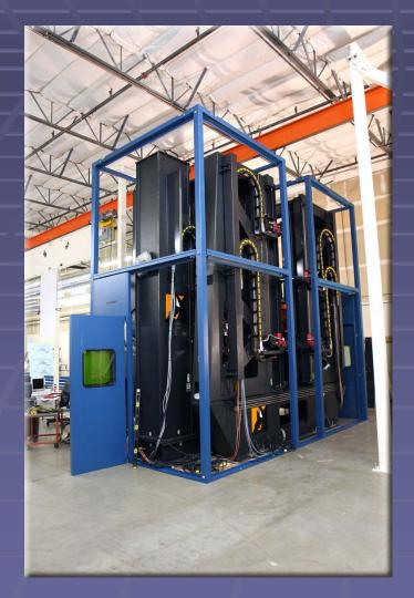
An overhead gantry transports wing skins through a fixed processing cell; the laser propagates ~150ft between the trailer and the cell.
