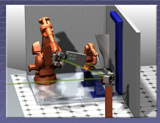
Mechanical design of the active beam delivery system (beam distances reduced for purpose of illustration)
