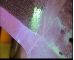
Figure 1. RHS Lower Fillet Crack Indication, Looking Aft and Up
