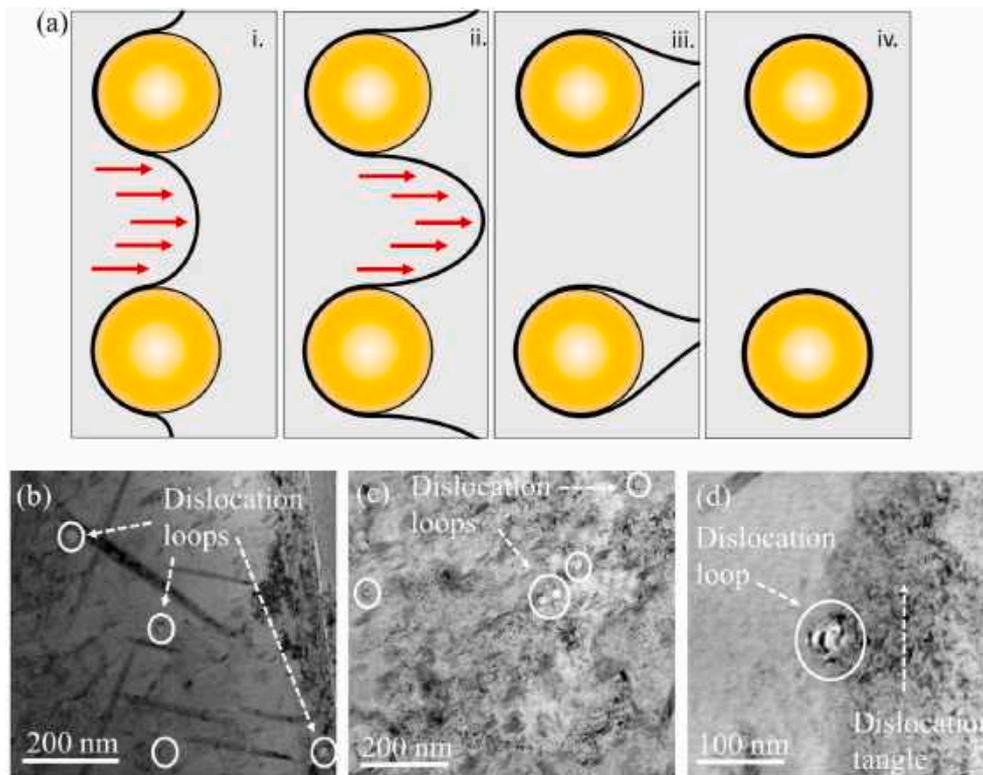
Fig. 7. (a) Schematic of dislocation movement during the Orowan bypassing mechanism; dislocation loops identified in AM-4LP-3HT-E at (b) the treated surface, (c) immediate sub-surface, and (d) an example of dislocation tangle forming behind a dislocation loop.
