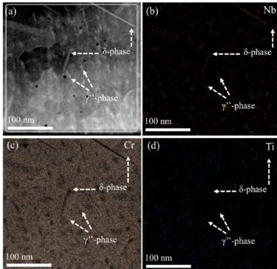
Fig. 2. TEM micrograph showing the presence of precipitated  $\delta$  and  $\gamma''$  phases, and respective EDX elemental maps showing (b) Nb; (c) Cr; and (d) Ti content taken from (a).
