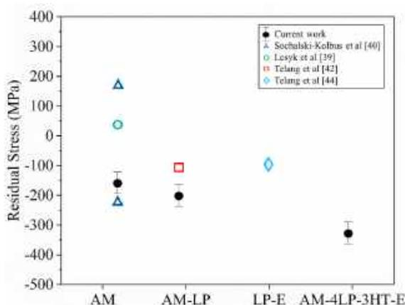
Fig. 3. Surface-level residual stress values of AM, AM-LP, and AM-4LP-3HT-E materials studied in this work alongside previous reports on surface-level residual stresses in as-built additively manufactured Inconel 718, Inconel 718 subject to a single LP shot, and laser peened Inconel 718 subject to a 24-h, 600 °C exposure (LP-E).
