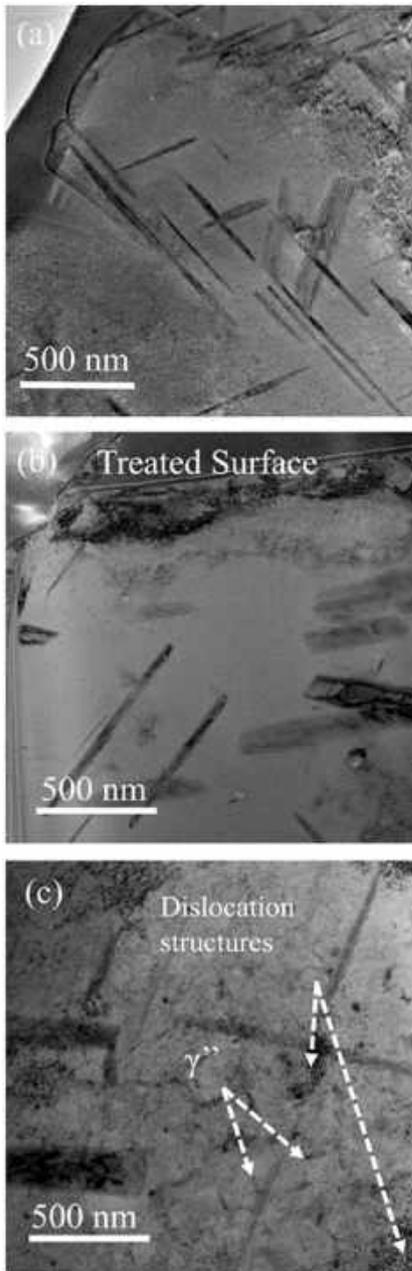
Fig. 5. TEM micrographs illustrating  $\gamma''$  content in (a) AM, (b) AM-LP, and (c) AM-4LP-3HT-E.
