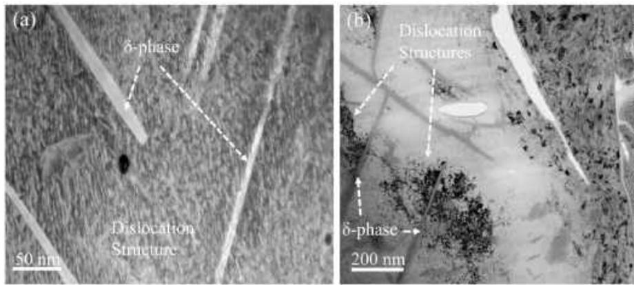
Fig. 6. Examples of  $\delta$ -phase precipitation pinning identified in (a) AM-LP and (b) AM-4LP-3HT-E.
