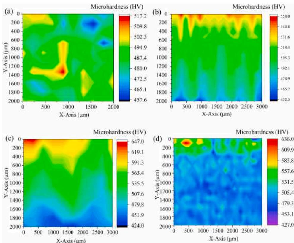
**Fig. 4.** Microhardness contour maps of (a) AM, (b) AM-LP, and (c) AM-4LP-3HT, and (d) AM-4LP-3HT-E specimens. Y-Axis represents the depth of the measured region while  $Y = 0$  represents the surface of the specimen that was laser peened; X-Axis represents the width of the measured region.
