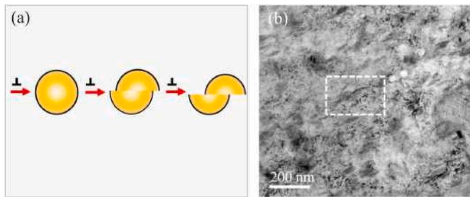
Fig. 8. (a) Schematic illustrating precipitate shearing, and (b) identified example of  $\gamma''$  shearing in the AM-4LP-3HT-E sample.
