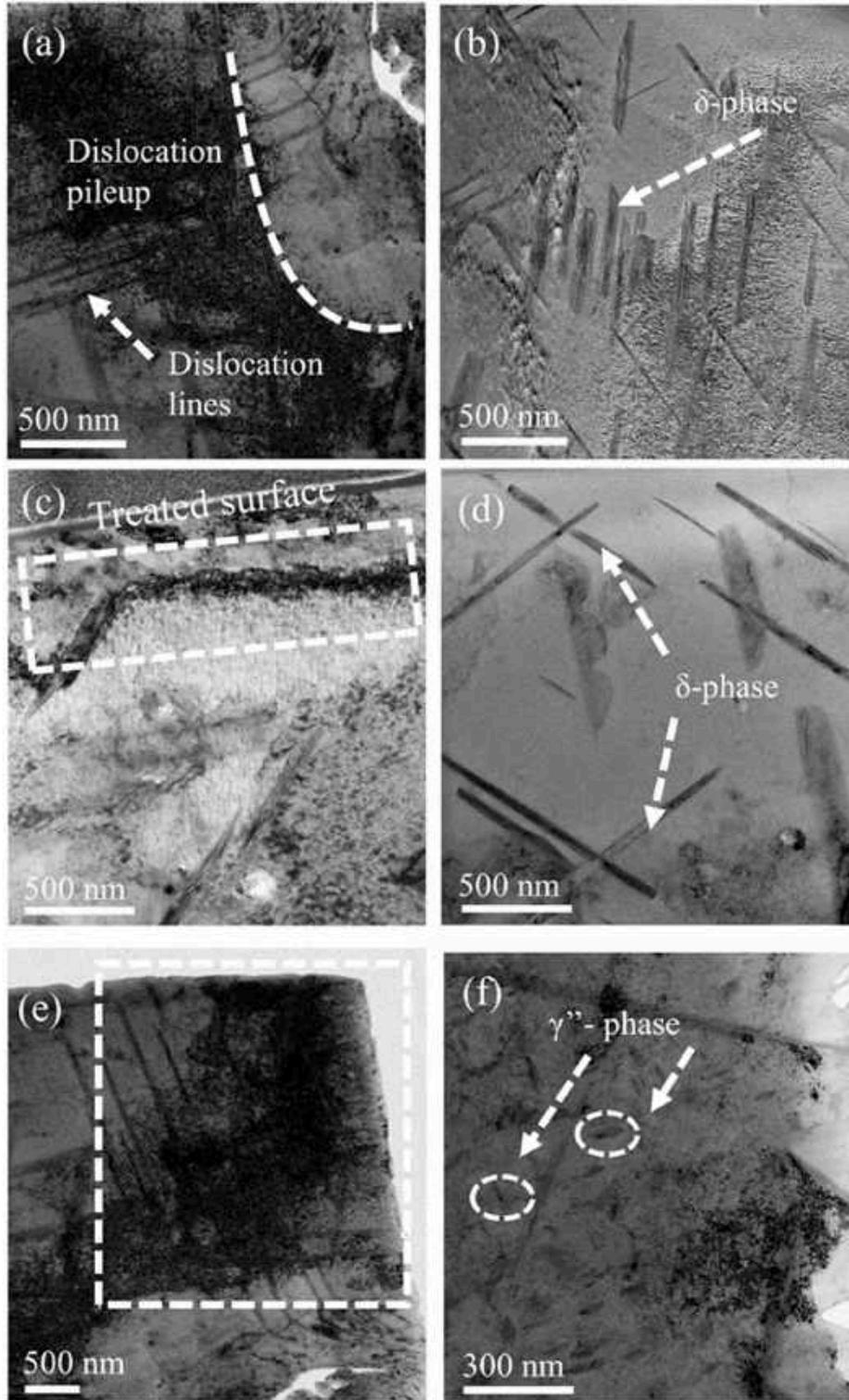
**Fig. 1.** TEM micrographs of (a) AM sample, highlighting the presence of highly dense dislocations, (b) presence of  $\delta$ -phase in the AM matrix, (c) presence of highly dense dislocations in the AM-LP sample, (d) additional evidence for intermediate phase formation, (e) large, surface-level dislocation network in the AM-LP-3HT-E sample, and (f) solid-state coherent precipitates discovered in AM-LP-3HT-E.
