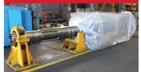
A work area that has been tented to protect facility and staff from flying media
