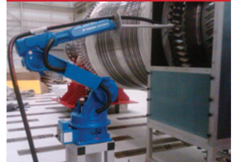
Programmable robotic peening
