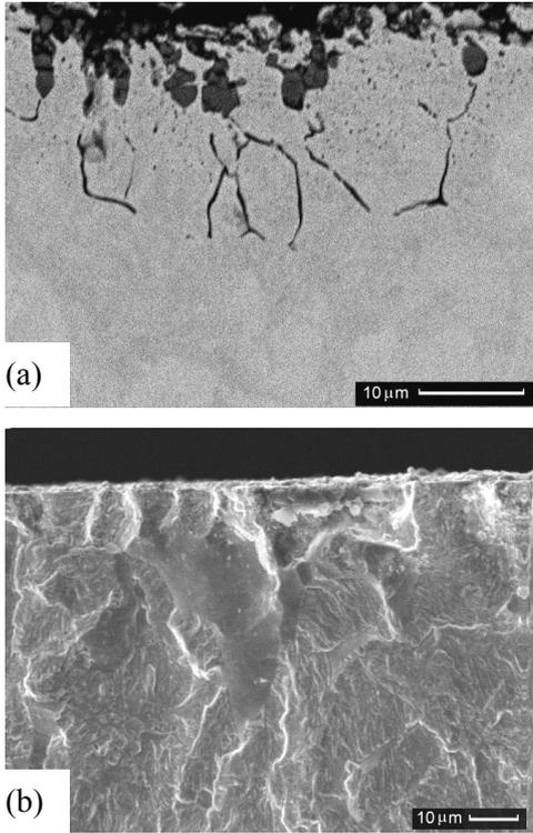
Figure 1 (a) Section with internal oxidation.
