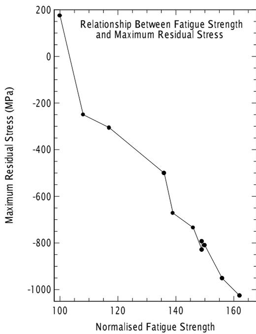
Figure 5 Relationship between residual Stress and fatigue strength.
