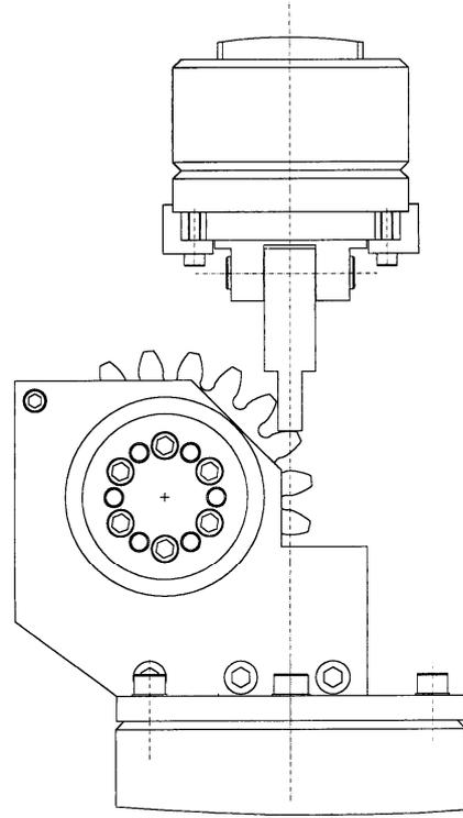
Figure 2 Gear pulsator test method.
