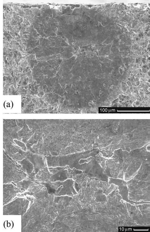
Figure 6 (a) Sub-surface initiation. (b) Nucleation from MnS.
