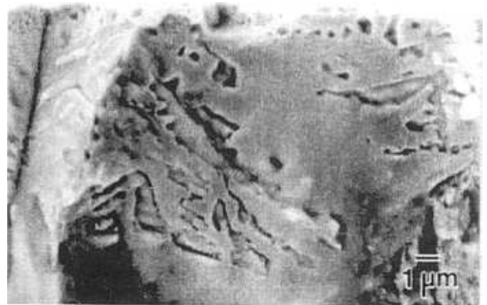
Figure 8. Oxide coverage on the intergranular fracture origin of a 0.6Mn-0.14Si modified 4320 Steel. SEM micrograph.
