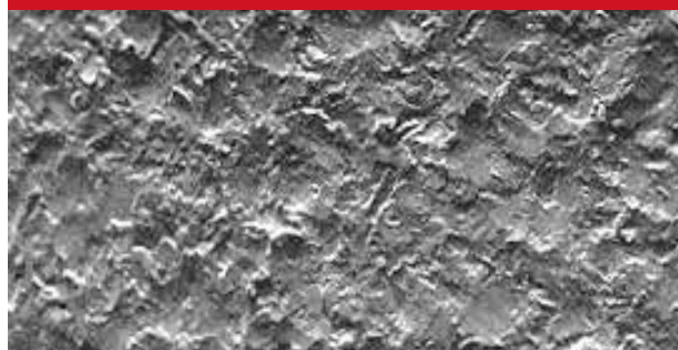
Fig. 10-13 SEM Photo of Dual Peen Surface Finish
