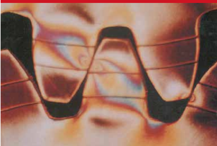
Fig. 4-3 Polarized View of Applied Gear Stresses
