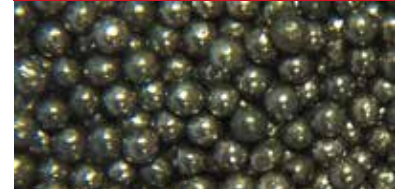
Fig. 11-3B Poor Quality Shot Peening Media
