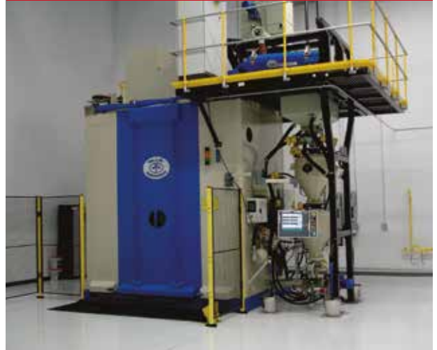
Fig. 11-10A Computer Monitored Lance Shot Peening Machine for Processing Internal Bores
