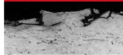
Fig. 11-2B Typical Surface from Proper Media
