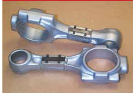
Fig. 11-6 Almen Strip Mounting Fixture
