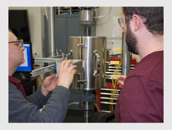
The team at IMR Test Labs performed fatigue testing and provided a series of S/n curves. After 60 samples, the test showed that the coating had the characteristics necessary to ensure success in its intended application.
