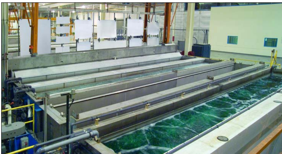
MIC's sulfuric acid anodizing line in Bensalem, PA features tanks measuring 40 feet long by 5 feet wide by 12 feet deep the largest SAA non-captive tanks on the U.S. East Coast.
