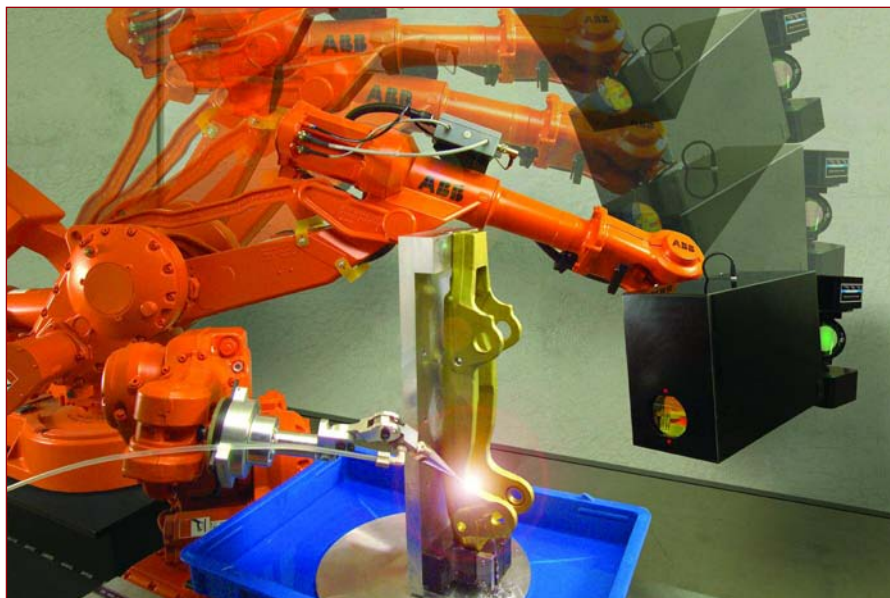
Figure 6. Moveable beam assembly comprising two electronically controlled, gimbaled mirrors and beam conditioning hardware allows movement of the peening laser beam over a stationary component such as an aircraft structure.
