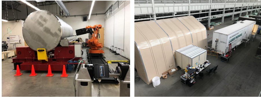
Figure 15. Laser peening system configured for treating welds of nuclear spent fuel canisters. At left beam director mounted on the robot (orange) for canister processing. At right system configured for field operation.
