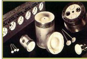
Typical Components coated with Thermal Barrier Coating (TBC)
