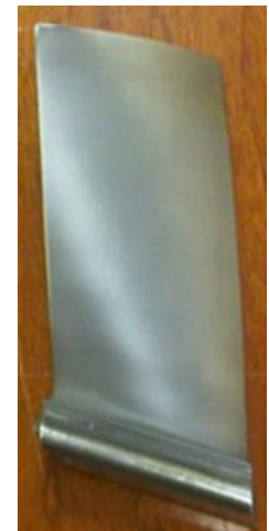
Iano-Smooth WC-CoCr coating ( Ra < 50 \mu\text{inch} ) on a Ti-alloy blade after polishing
