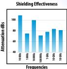
The above shielding effectiveness data applies only to three of E/M's conductive coating processes.
