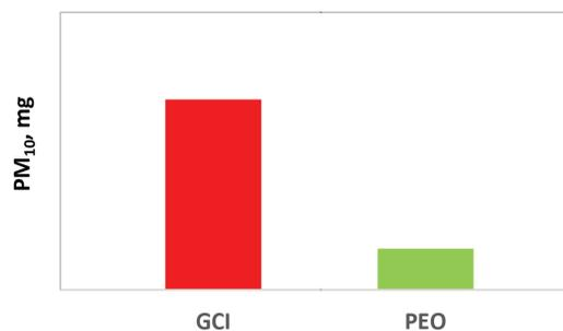
Fig.4. Decrease in PM<sub>10</sub> emissions by 78% for PEO-Al compared to GCI (Courtesy: Fabian Limmer PhD work at the University of Leeds).
