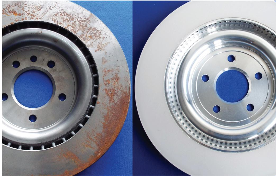
Fig.1. GCI disc (left) and PEO-Al disc (right).
