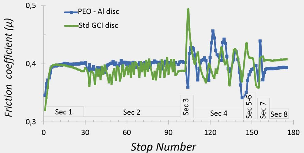
Fig.3 Average CoF values of PEO/Al disc vs GCI disc at 100°C IBT during AK Master test.
